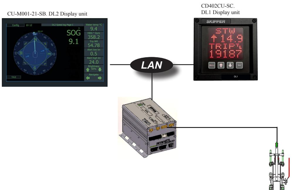
*The DL21 Speed Log is designed for ships over 50.000 GT with simultaneous and independent measurement of speed through water and speed over ground to comply with the requirements of MSC.334(90), amendments to performance standards for devices to measure and indicate speed and distance.*
